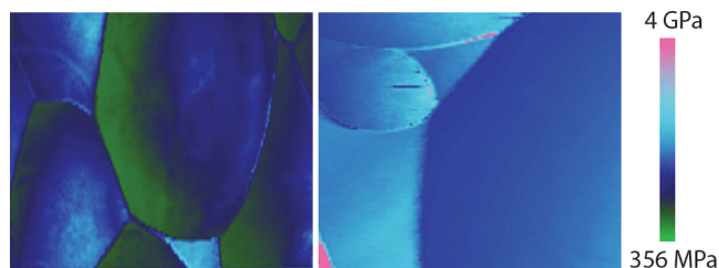
Figure 5. Representative E-Modulus images of the PLLA particles (left) and the SC particles (right) used as fillers (AFM PeakForce QNM). All QNM images were scanned over an area of 1 \times 1 \mu\text{m} .
